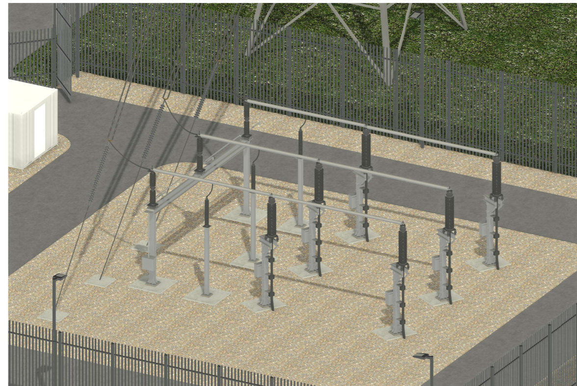
CABLE SEALING COMPOUND (LEFT COMPOUND) 3D VIEW
